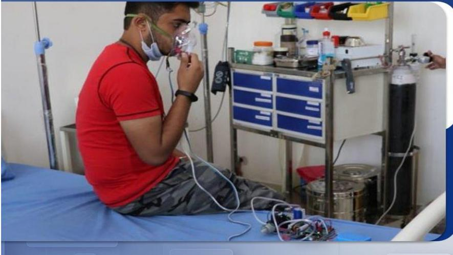
To increase the life of medical oxygen cylinders three fold, the IIT, Ropar has developed a first-of-its-kind Oxygen Rationing Device – AMLEX that supplies a required volume of oxygen to the patient during inhalation and trips when the patient exhales CO<sub>2</sub>. This process saves oxygen which otherwise unnecessarily get wasted.
