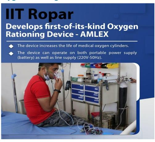
To increase the life of medical oxygen cylinders three fold, the IIT, Ropar has developed a first-of-its-kind Oxygen Rationing Device – AMLEX that supplies a required volume of oxygen to the patient during inhalation and trips when the patient exhales CO2. This process saves oxygen which otherwise unnecessarily get wasted.
